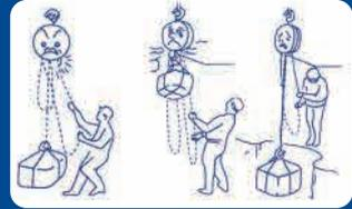
No hook tip loading. No direct binding of a load with a load chain.
