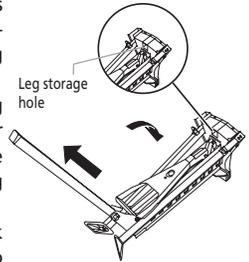
**NOTE:** when transporting the work station, the rear leg becomes the carrying handle.
