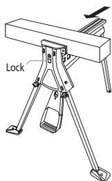
**NOTE:** When clamping long or heavy materials, always provide proper support for the work-piece.
