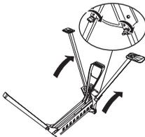
**⚠ CAUTION:** To reduce the risk of injury, never attempt to lift the work station until the rear leg has been properly secured in place.
